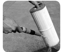
Hose off cleaning solution
